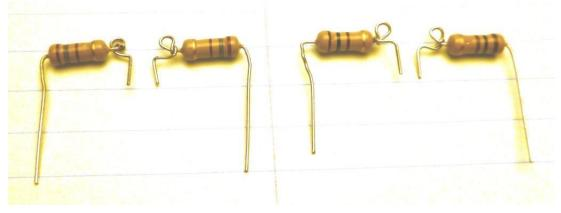
4. Insert the  $180\Omega$  resistors in positions R2 (two places) with the looped ends positioned as shown below, solder and trim the leads.
