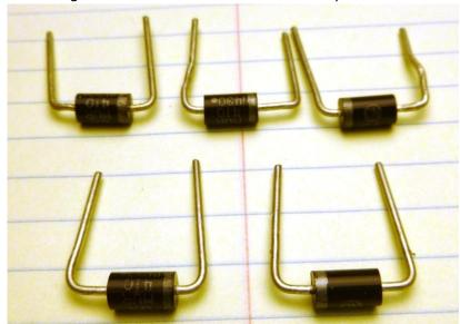
23. Assemble to the board with the white banded ends orientated as marked by the arrows in the picture below. Space the diodes 2 to 5 mm above the board.
