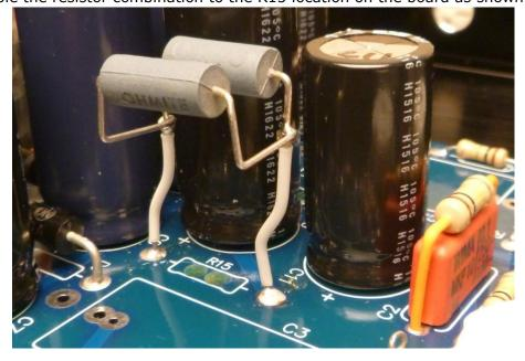
35. NOTE: C3, two places, (the output caps) will be assembled to the board after the initial voltage tests.
