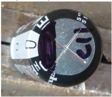
28. Assemble caps C10 and C11 to their respective places on the board, ensure they resemble the picture below, solder and trim the leads.
