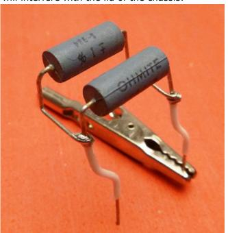
34. Assemble the resistor combination to the R15 location on the board as shown below.
