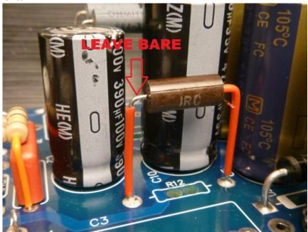
33. Connect the two 51 ohm 3 watt resistors (Mouser part no. 660-MOS3CT631R510J) in parallel as shown below. Use some stripped-off insulation to cover the leads as these resistors will sit quite high above the board, again for heat dissipation. Note: Once installed the resistors are <u>not</u> to rise above the level of the tallest filter capacitors or they will interfere with the lid of the chassis.
