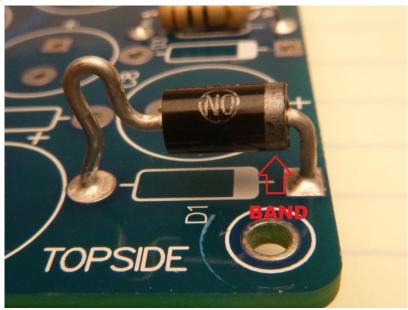
22. Prep all 5 remaining MUR 410 Diodes as shown in the picture below.
