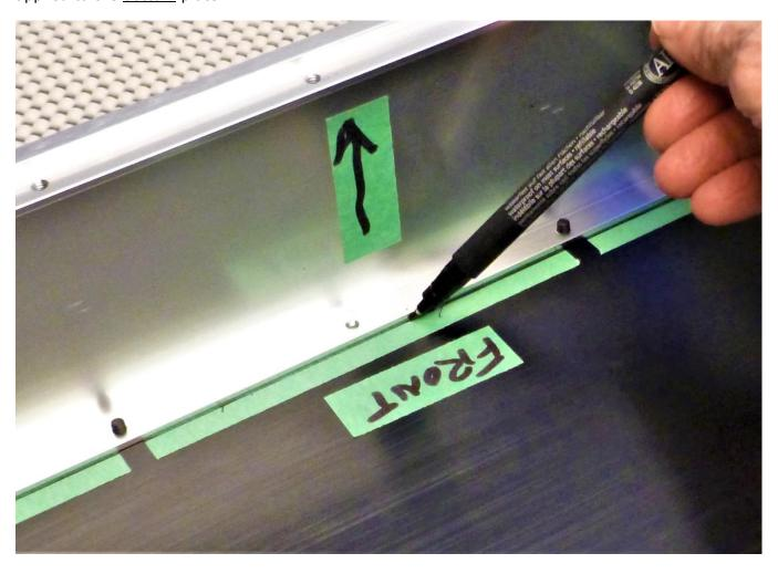
Label the  $\underline{right}$  side of the bottom plate for the power supply board, the  $\underline{left}$  side for the amplifier board as shown below.
