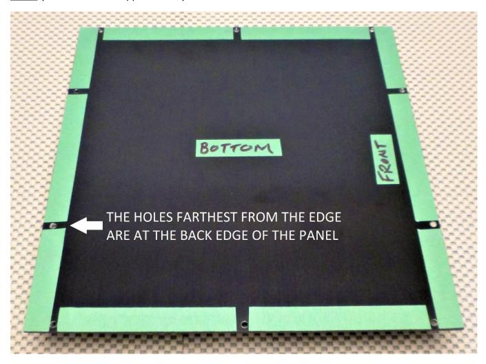
Attach the  $\underline{\text{back}}$  panel to the  $\underline{\text{bottom}}$  panel with the AC inlet hole on the  $\underline{\text{right}}$  side as viewed from the front. Leave the screws slightly loose.
