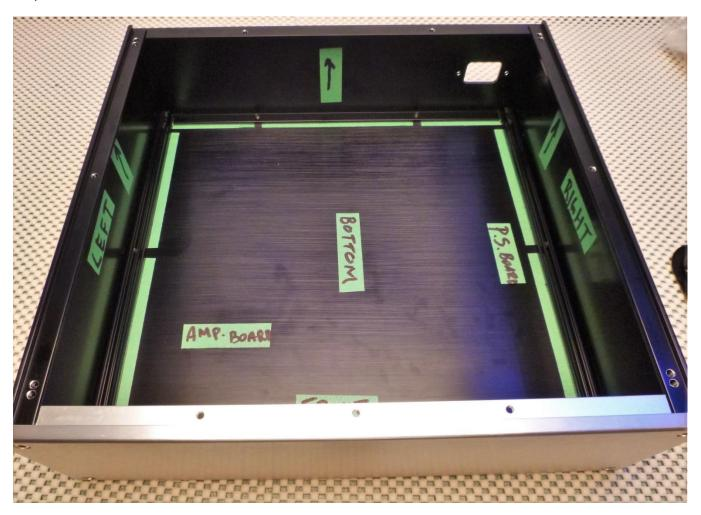
Remove the bottom plate from the sides, front and back.
