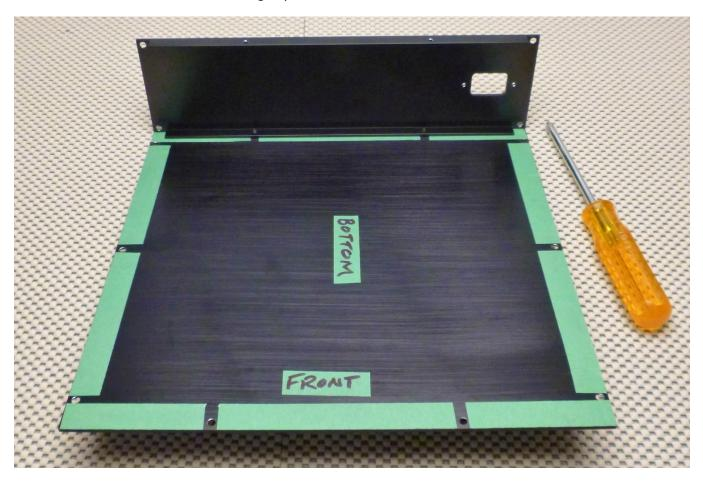
Note: The  $\underline{\text{side}}$  panel upper and lower "rails" have an inset on one end. These ends connect with the  $\underline{\text{rear}}$  panel of the chassis.
