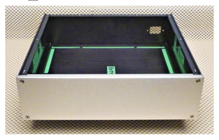
Attach the  $\underline{\text{top}}$  and tighten all screws.
