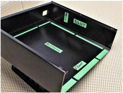
Attach the <u>front</u> to the bottom and sides but leave the screws a little loose.
