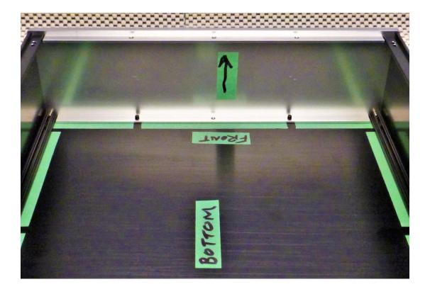
Using a fine point marker, draw a line around the inside perimeter on the tape previously applied to the  $\underline{\text{bottom}}$  plate.
