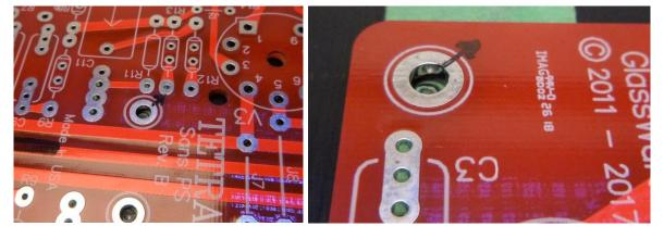
When happy with the centre punch locations, centre drill, then drill the remaining holes with a 1/8" (or 3.2 mm) drill. Deburr the holes.
