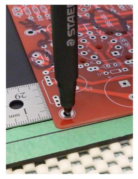
Alternatively, use a centre punch, automatic punch or transfer punch of appropriate size to mark the position of **one** corner hole as shown. Note: Transfer punches are for making light indentations only. Just tap them lightly then use a centre punch to make a deeper indentation.
