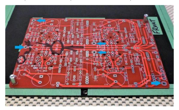
Mark the positions for the remaining 5 holes as shown above. Remove the board. Centre punch, then put the board back on the two holes already drilled. If any centre punch marks need to be "moved" as described earlier, do this before drilling. This is a pain but it's a lot easier than filing holes that are slightly displaced from the ideal position.
