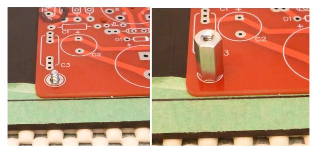
Align the opposite end of the board with the line drawn on the tape or align it so that it's a consistent distance from the line over the length of the board. If you have a scared-up work bench like mine a recess can usually be found (or made) for the head of the 4-40 screw protruding below the bottom panel.
