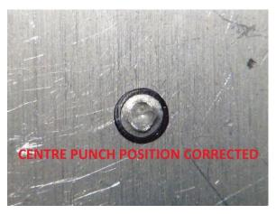
Once you think you have the centre punched hole in the correct location put the board back on the bottom and check as before. As above, remove the board, centre drill, then drill a 1/8" (or 3.2mm) hole and deburr.
