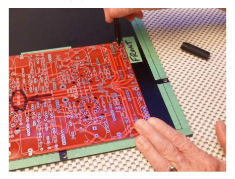
Use a light and check the hole location on the bottom panel relative to the hole on the board.
