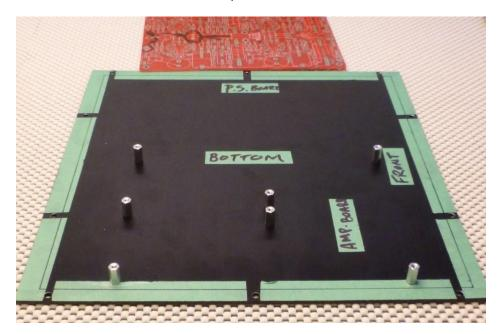
Place the board, top side up, input to the rear, over the spacers then thread seven 4-40 screws through the holes in the board into the spacers to check that they all fit. If you've been careful in your layout and drilling you won't have to file any holes in the bottom plate. <u>Don't</u> file the holes in the circuit board.
