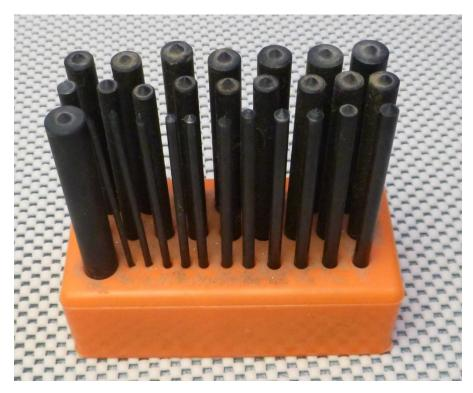
If you don't want to buy a variety of punches a fine tipped marker and one centre punch will work well. That's what I used for this project. It's a bit more work but with patience and care the holes in the bottom plate lined up with the standoff holes in the circuit board without any filing needed.
