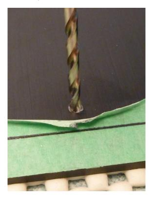
After the hole has been drilled deburr both sides with the small countersink turning at a <u>very slow</u> speed in your power drill.
