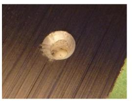
Using a 1/8" (3.2 mm) drill bit, (start slow then increase speed) drill a hole at the centre drilled location. When drilling aluminum a few drops of alcohol (methyl hydrate) on the drill bit will help keep it cool and cutting better.
