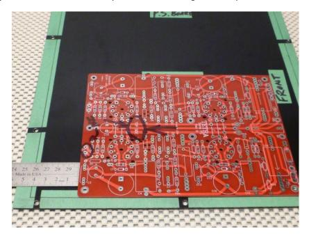
Set the edge of the amp board along the line on the tape as shown below. Don't be concerned that the board is too close to the edge. When it is mounted on the board spacers it will clear the side.
