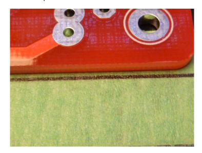
On a hole in the opposite corner of the board centre punch, transfer punch or if your punches are too big to fit through the hole, mark its position with a felt tipped pen. Use a piece of tape underneath if it helps you see the hole location.
