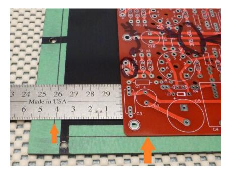
If you don't have a centre punch that fits the standoff holes in the board precisely use a fine tipped marker to mark the hole.
