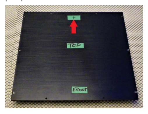
Place the top panel to your bench with the outside (side with countersinks facing up) and the just-drilled hole farthest from you.
