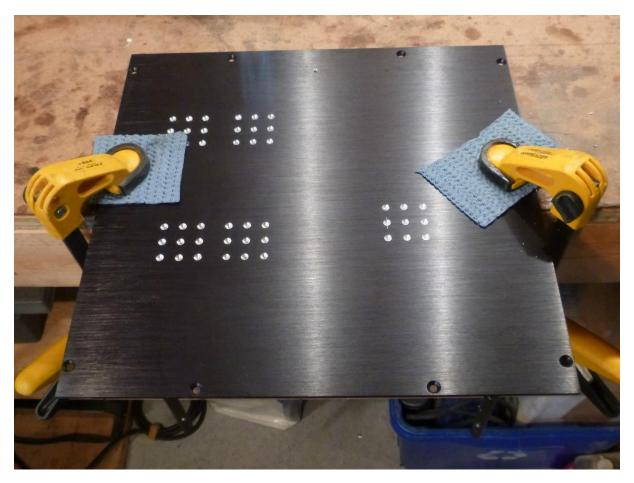
If using a hand-held drill, it's near-essential to clamp the panel to your work bench as the larger drills tend to "grab" when drilling. Put a piece of rubber between the clamp and the panel to protect from damage.
