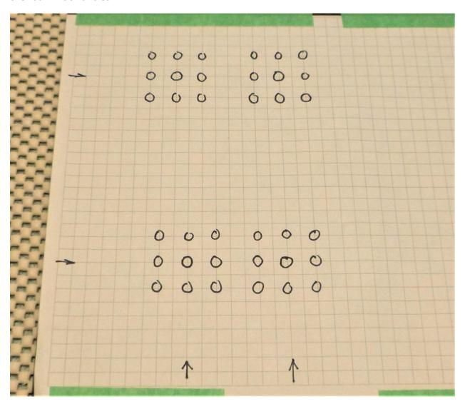
Measure over 3 5/8" (92mm) from the right-hand edge and put a mark on the line nearest.
