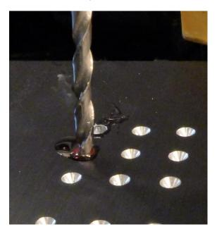
With the drill bit <u>not</u> turning place it in the centre-drilled recess. Start the drill turning slowing then increase speed once it has started to "bite" into the panel.
