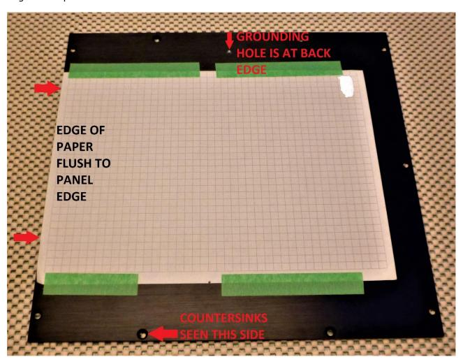
Measure over 2 1/2" (63mm) from the left-hand edge and put a mark on the line nearest. Measure over 4 3/8" (111mm) from the left-hand edge and put a mark on the line nearest.
