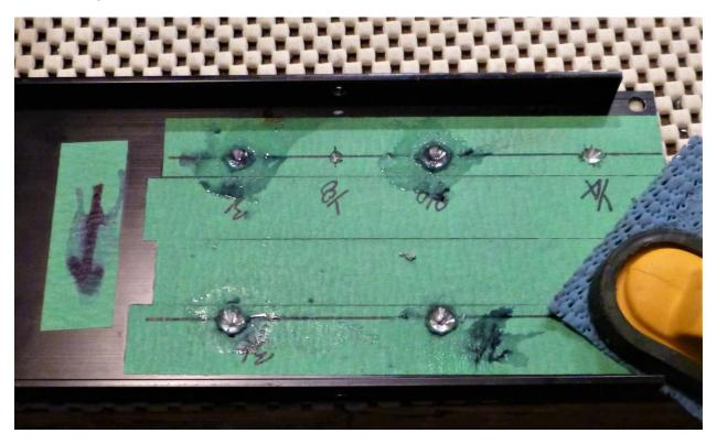
Centre drill the 6 holes. At the 1/4 and 3/8 locations allow the angled part of the centre drill to bite into the panel as shown above. This will help guide the drill bit.
