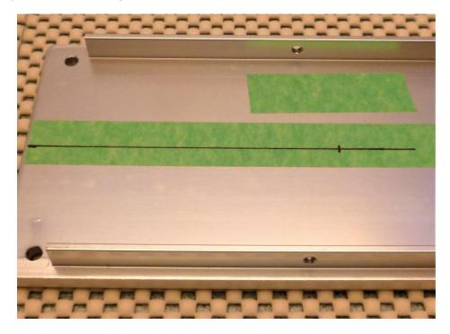
Draw a vertical line up from the position just marked. A small piece of scrap metal or wood that has two adjacent side square will aid in layout.
