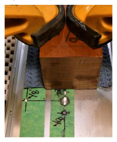
Drilling a large hole with a hand drill can be difficult. Drill through the plate with a 1/4" (6.4mm) drill first. Use the larger countersink to put a small bevel on the 1/4" hole then drill with the 13/64" (9mm) bit.
