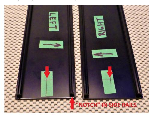
Center punch, centre drill, drill a 1/8" (3.2mm) hole and deburr, one hole in each side panel.
