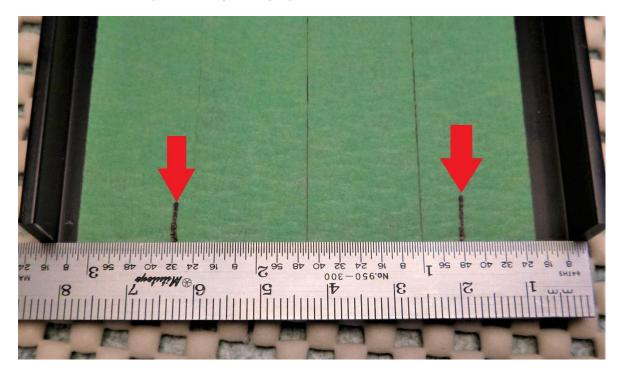
Using a square draw lines across the tape on the marks made above.
