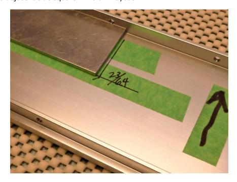
Measure up 1 3/16" (30mm) from the 23/64 position and mark. Write 1/8 near this location.
