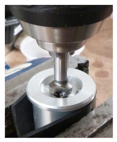
Put a 1/4" or 6.4mm drill bit in your drill and dip the end in ATF.
