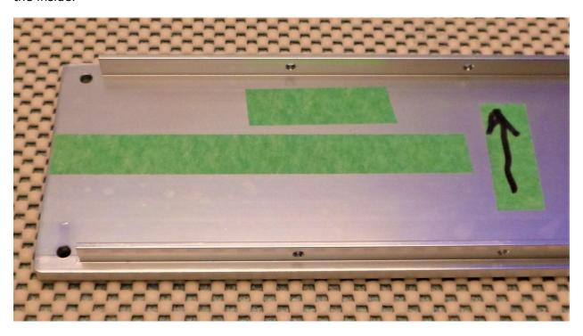
Measure up 1 13/16" (46mm) see, isn't metric easier, from inside the bottom edge of the panel and put a mark on the tape.
