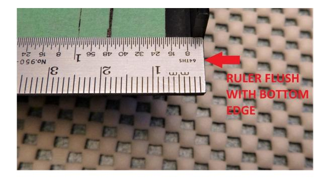
Place a mark on the tape 3/4" (19mm) up from the bottom.
