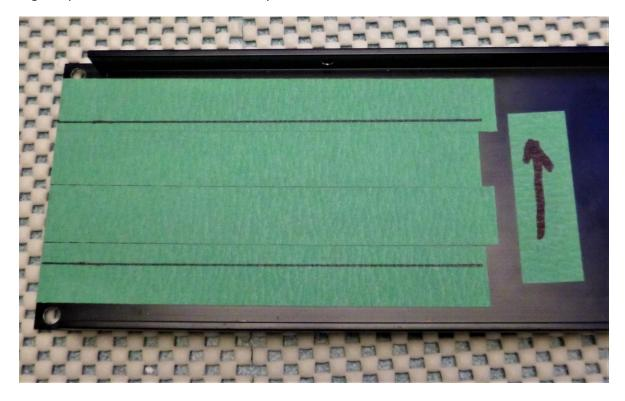
On the lower line measure over from the left-hand edge 3/4" (19mm) and mark the position. Write 1/4 close to the mark. See below.
