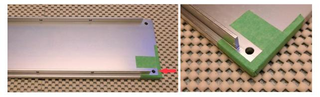
Once the masking is complete use the corner of a ¼-sheet palm sander with 150 to 220 grit paper and sand until bare aluminum can be seen. It will be a bit harder to see on the back of the natural anodized front panel. Usually only a few seconds is required to remove the anodizing.
