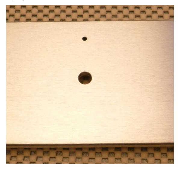
As before put the <u>minimum</u> chamfer on the two 1/8 (3.2) holes just drilled, especially on the "top" one where it pierces the <u>outside</u> of the panel. Just twirling the small countersink in your fingers might be sufficient.
