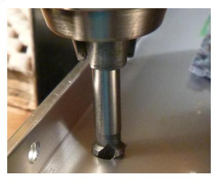
Using the large countersink, keep taking small amounts of material out then checking the depth with the LED specified in the parts list. The depth of the countersink should be such that at the proper depth the front face of the LED should be flush with the front of the panel. It will appear quite recessed from the back as shown below.
