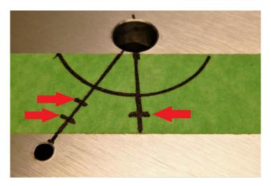
On the vertical line between the large hole and the LED hole, 5/32'' (4mm) out from the traced circle, place a mark on the line. See above.
