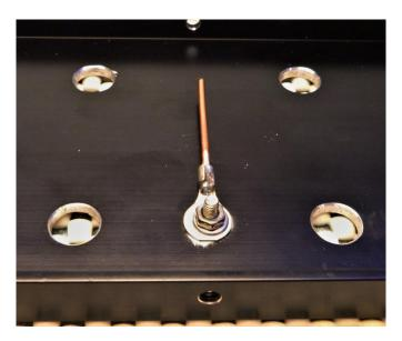
Wipe the inside of the right-side panel (the one with the long ground wire). Assemble two of the cable tie mounts near the top edge in the positions shown below.
