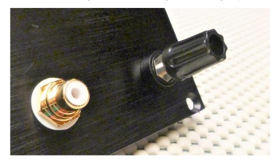
Put the remaining plastic washer, the metal flat washer and a nut on the shaft and tighten. The solder lug and second nut will be added later.
