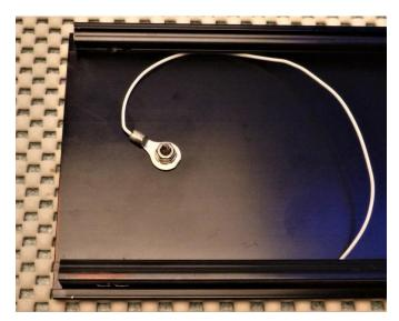
Cut a piece of wire 14" (36cm) long, strip one end and solder to part no. 534-7311 lug.
