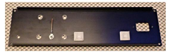
Assemble the AC inlet to the rear panel with the ground terminal (marked E) closest to the bottom edge as shown below. Put a drop of nail polish on two screws and secure the inlet to the panel.
