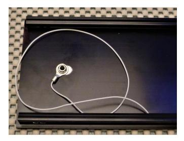
Cut a piece of wire 10" (25cm) long, strip one end and solder to part no. 534-7311 lug. Set this aside it will be connected to the top later.
