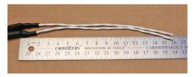
Strip  $1\frac{1}{4}$ " (30mm) of the cable sheath from the ends.
