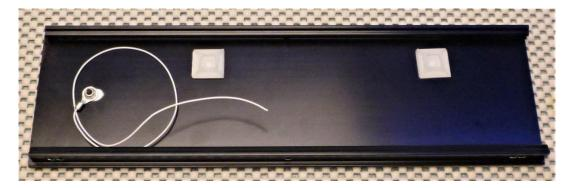
Wipe the inside of the left-side panel (the one with the short ground wire). Assemble two of the cable tie mounts near the top edge in the positions shown below.
