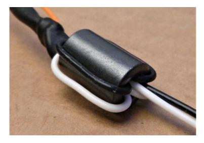
Measure back from the ferrite 19" (48cm) and cut the cable or twisted pair.
