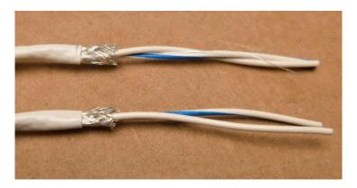
Strip about 1" (25mm) of insulation off of two 3" long pieces of wire.
