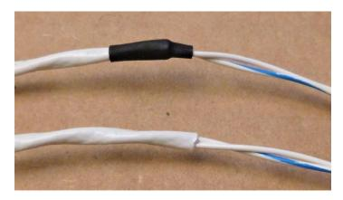
I've shown one with heat shrink tubing above and one without for visual purposes. You will of course cover both with heat shrink in this and subsequent cable assemblies.
