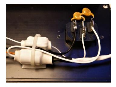
Prepare two of the following cables that will go from the input jacks to the amp board.
