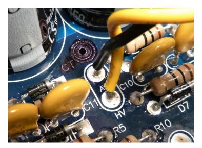
Insert the red-yellow pair from the filament transformer into pad **A** and the black-orange pair into pad **C** on the power board and solder.
