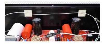
Strip the front grounding wire, the left-side grounding wire and the one made earlier for the top panel grounding. Connect to the copper grounding bar and solder. Secure with zip ties, see below.
