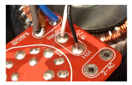
Connect and solder the leads from the B+ transformer to the **2-AC** pads on the switch board as shown below.
