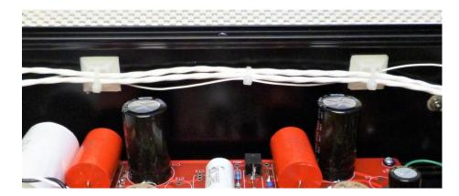
Cut the cables so that when they are formed around the side and back of the chassis they go past their respective jacks by about 1'' (25mm), see below.
