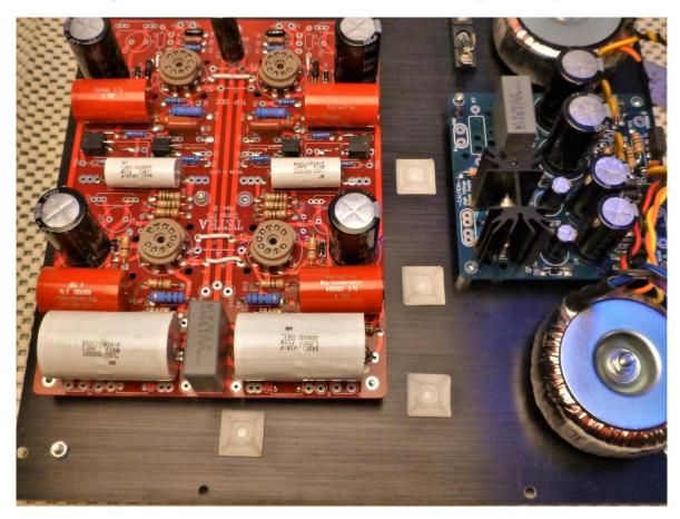
With an alcohol dampened paper towel wipe the bottom panel between the two boards and in front of the amp board.
