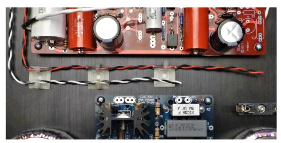
Strip the wires from the H+ and H- on the amp board, black and white in this instance. Connect to the H+ and H- on the power supply board. Before soldering ensure that the H+ on the amp goes to the H+ on the power supply and the H- on the amp goes to the H- on the power supply.
