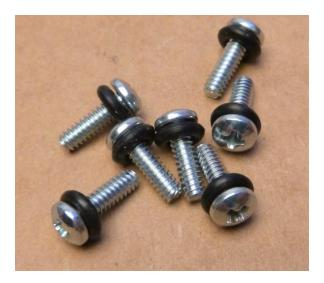
Position the amplifier board on the bottom panel aligned with its standoffs. Put a drop of nail polish on the threads each screw. Start them through the board into the standoffs.
