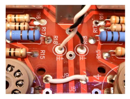
Cut two lengths of shielded cable (a twisted pair of hookup wire is OK) 28" (70cm) long.
