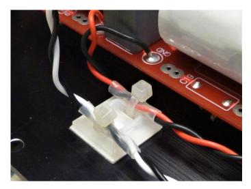
Form the wires over the other three cable tie mounts, shrink the tubing into position and strap with zip ties as shown below. Cut the wires to the length shown.
