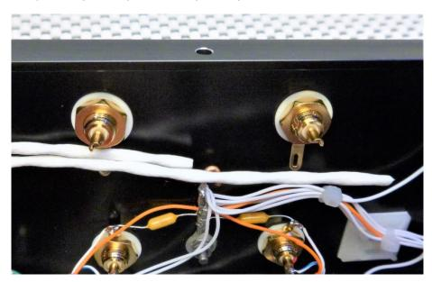
Remove about 1" (25mm) of jacket and shield, or just strip the ends if you are using twisted pair wiring. Slide a short piece of heat shrink over the cable. Strip the ends and solder as shown below. Make sure you connect the lead on the + end back at the amp board to the centre pin of the RCA jack. See below.
