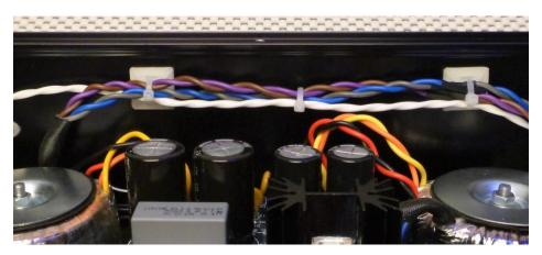
Trim the cable from the AC inlet to about the same length as the B+ transformer leads. Remove 1'' (25mm) of sheath and shield (if you are using shielded cable) and put a piece of heat shrink on the end as shown below. Strip about 3/16'' (5mm) of insulation from the wires.
