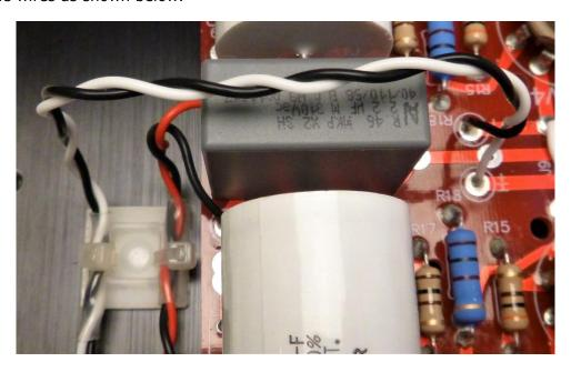
Slide the heat shrink tubing into position on the wires and heat. Strap to the cable tie mounts with zip ties as shown below.
