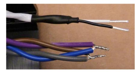
It's easier to connect the wires to the power switch before it's assembled to the front panel.
