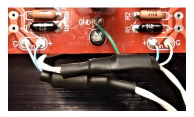
Secure the leads from the board to the output jacks to the right-side cable tie mounts as shown below.
