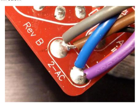
Strip a bit of insulation off of the free end of the ground wire connected the **GND** pad at the back of the circuit board. Solder to the lug that came with the binding post. Assemble to the binding post and secure with the nut. Lock the nut in in place with nail polish on the nut and thread. See below.
