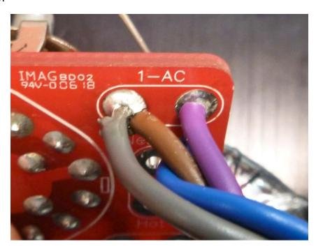
Connect the power lead from the **neutral** on the AC inlet, white in this instance, to the **Neutral** pad on the switch board. Connect the other lead to the **Hot** pad on the switch board and solder both.
