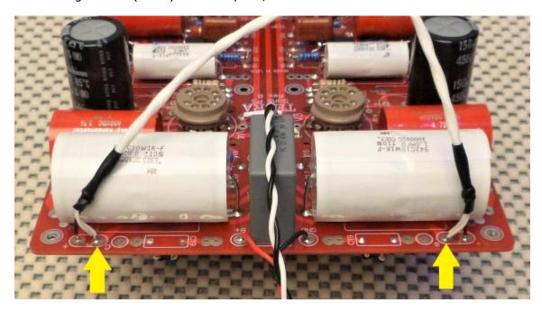
Cut a 6'' (150mm) piece of wire, strip one end, and solder to the **GND** pad at the input end of the board.
