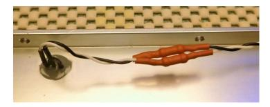
Cut a piece of wire about 24" (60cm) long, strip one end and solder to the **House** ground on the power supply board.
