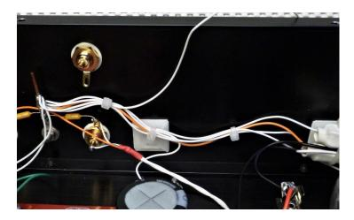
Strip the leads coming from the ferrite noise filters on the input cables. Connect the "hot" leads (the ones connected to the centre pins of the RCA jacks) to the + input pads. The other leads connect to the G (ground) pads. Solder the leads as shown below.
