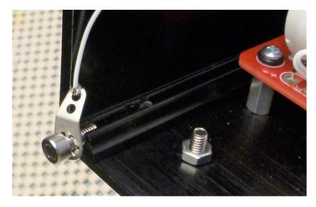
Run the wire through the cable anchors, see below.
