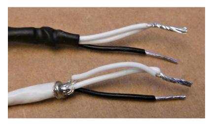
Cover with heat shrink tubing as shown above.
