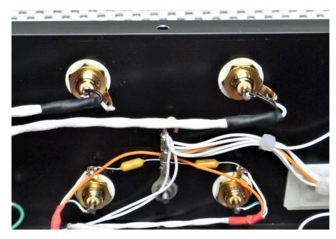
Tighten the nuts securing the output jacks. Apply a drop of nail polish to the nut and thread of all four jacks.
