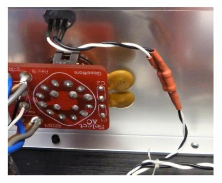
Route the wires from the LED along the filament wires from the amp board and secure with dental tape or zip ties. Cut to length and strip the ends. Solder the wire from the **centre** pin of the LED to the spare **H**- pad on the power supply board. Connect the other lead to the spare **H**+ pad on the power supply board.
