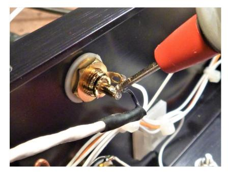
Turn the amplifier off and disconnect the multimeter negative lead from the ground. Leave the grounding plugs in place.
