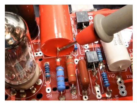
Lastly check the AC and DC voltages on both output jacks as shown below. In either case it should measure well under 1/10 of a volt and likely much less.
