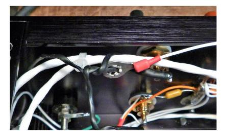
The B+ power leads from the amplifier board will be connected to the power supply board after initial testing.
