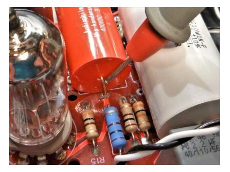
Measure the voltage after the second filter by touching the **positive** probe on the inboard ends of capacitors **C4**, one on each channel, as shown below. The voltage should be about 215 volts on the standard version and 280 volts on the alternate version.
