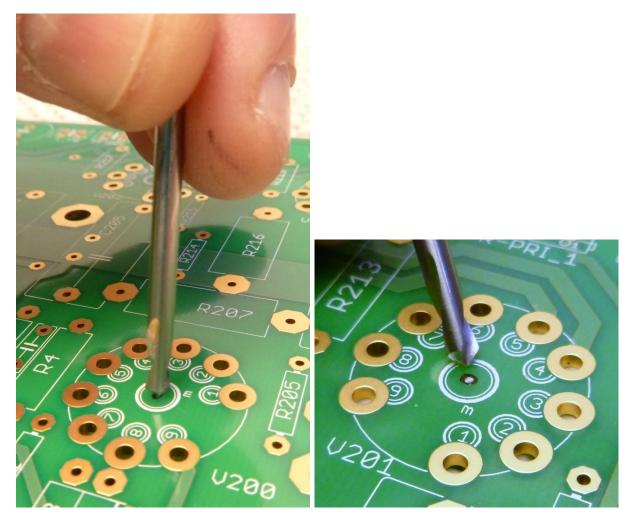
Twisting the centre drill in your fingers, lightly mark the board in the **seven** tube socket locations. This will make it easier to find the correct position when using the power drill.
