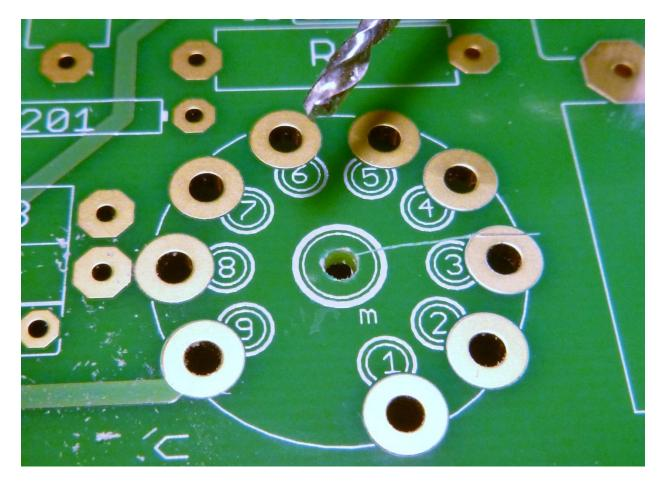
Chuck the 1.7mm or 1/16" bit and drill through the board in the seven marked locations.
