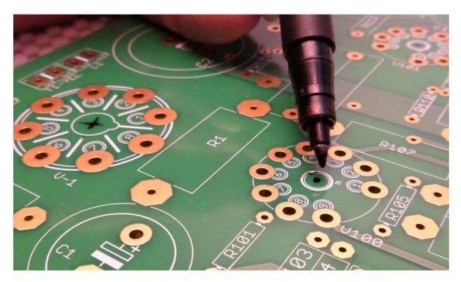
Mark the centre of each of the **seven** tube socket locations with a fine tip marker.
