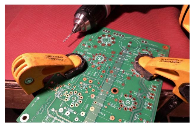
Clamp the board to the edge of a bench or table as shown.
