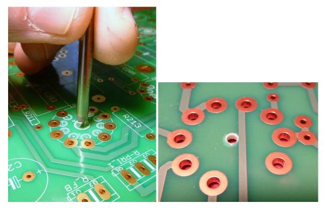
Use a small countersink to remove any burrs from drilling. Spinning it in your fingers should be adequate. Don't damage any PCB traces.
