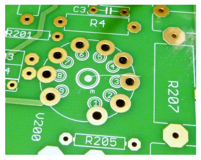
Chuck the centre bit in the drill. Set the drill speed to the slow setting. Drill the **seven** places at the locating mark to no larger than 1.7mm or .060" in diameter.
