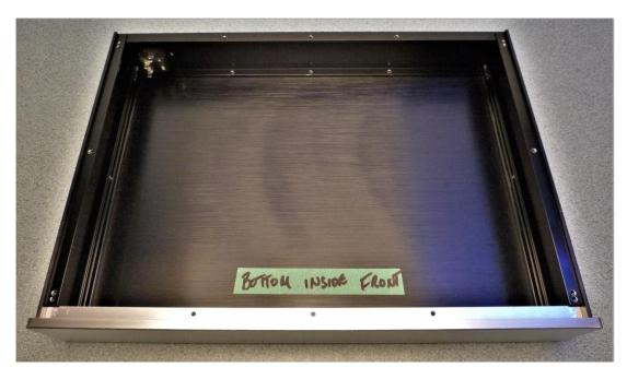
Remove the top, the AC inlet should be on the left side as shown above. If not remove the rear panel and rotate 180 degrees.
