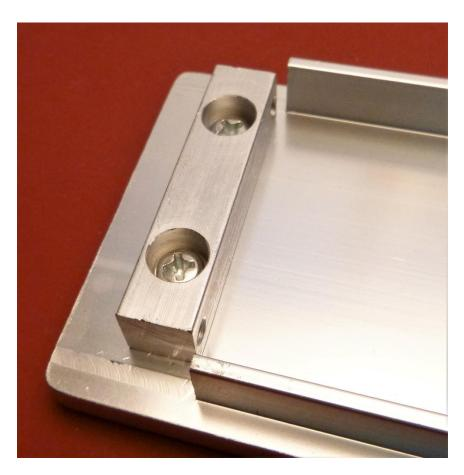
Assemble the **two** small blocks to the inside of the front panel but leave the screws slightly loose.
