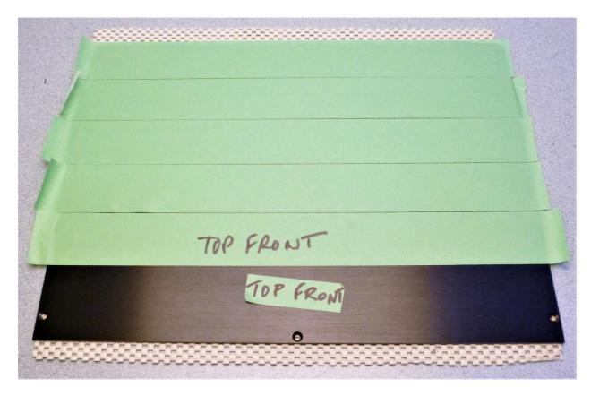
Cover the outside of the top plate with painters' tape. Be sure to label the front.
