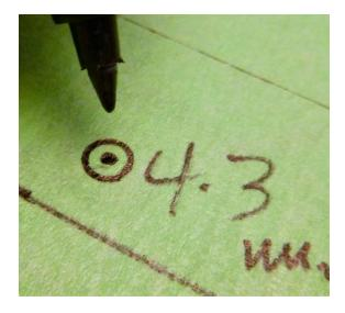
Mark a dot in the center of the circles designating the **five** board spacer locations and write **4.3mm** beside each (the drill size used later).
