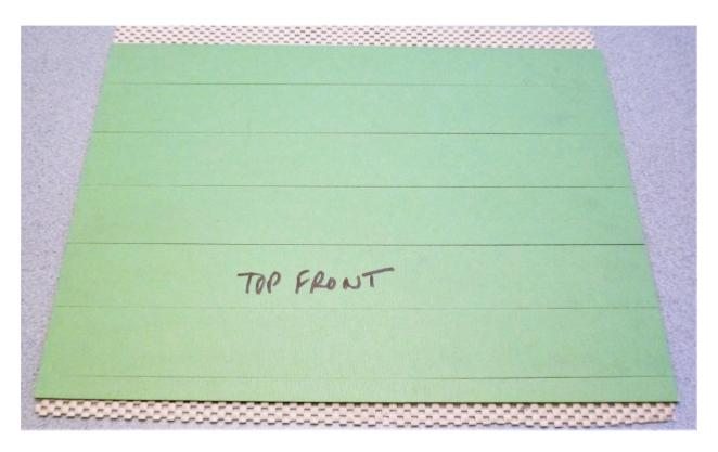
Trim the tape flush with edges of the top panel, being careful not to scratch the external surface of the plate.
