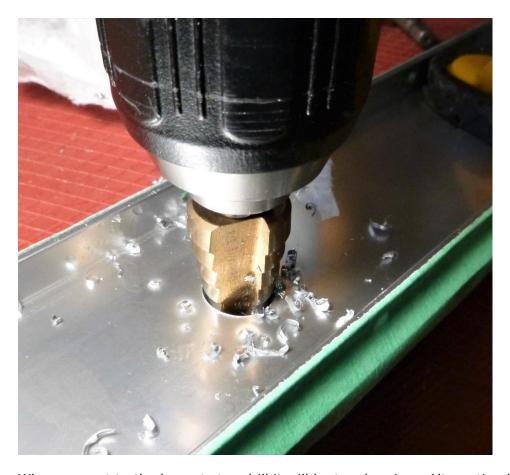
When you get to the largest step drill it will be tough going. Alternating between drilling from the front and from the back will help.
