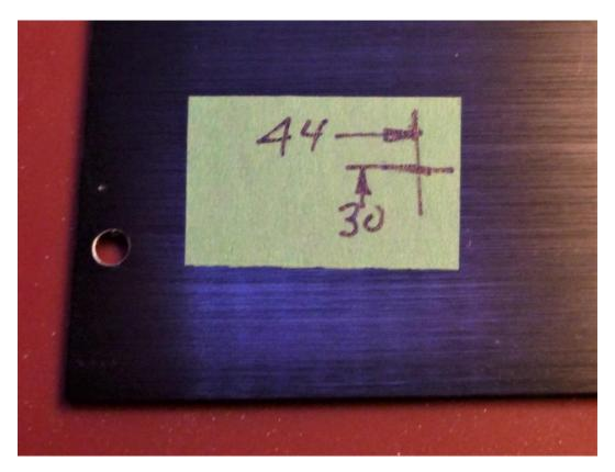
Measure and mark in 44mm from the sides and 30mm in from the top and bottom. Centre punch, centre drill and drill through the bottom panel with a 4.3mm (or 11/64"), bit. Remove the tape and deburr the holes with a countersink.
