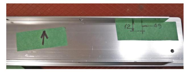
Place the panel in front of you with the inside facing up and the top edge away from you. This means that the left side, as seen from the outside, will be on your right.
