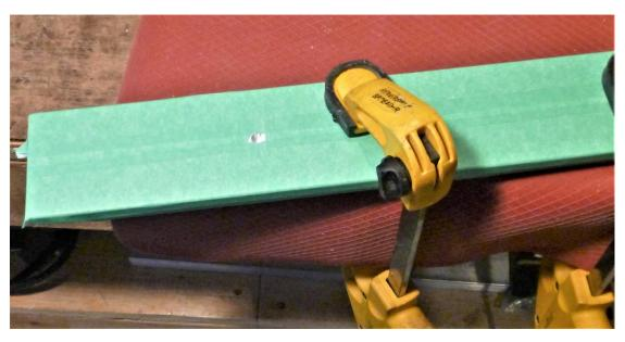
Centre punch and centre drill the spot. Cover the front with tape to protect it while drilling.
