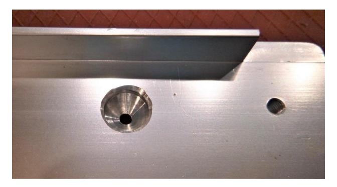
Using a 3/8" countersink cut your way down into the 3.1mm (or 1/8") hole drilled previously.
