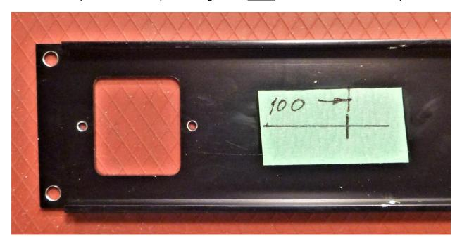
Apply a piece of tape as shown, draw a line centered between the top and bottom and another 100mm in from the left edge.
