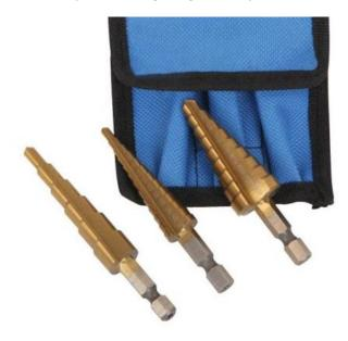
A sheet metal step drill set, like the one shown above is used to make a large diameter hole. These can be fairly expensive but I bought the set you see above at an automotive discount store for about \$15 on sale. Alternatively, 19mm (3/4") hole saw will make the require hole.
