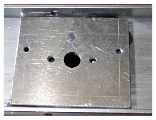
Epoxy applied and hole in plate aligned to hole in front panel. Set this assembly aside for several hours to give the epoxy a chance to fully cure.
