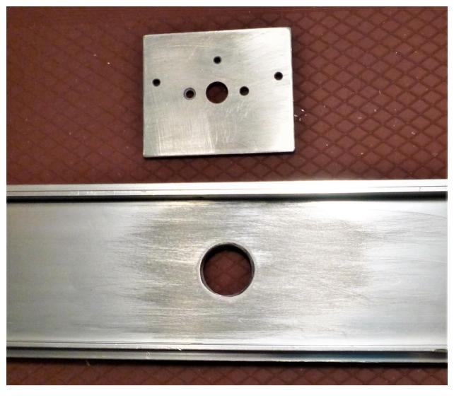
The 1/8" (or 3mm) plate used to mount the volume pot is shown just above the front plate. Both have been sanded lightly to give the epoxy used to stick them together a better grip. Note: There are 3 extra holes in the pot mounting plate not shown on the drawing in attachment 5. They are not required. This was a scrap piece and the extra holes were pre-existing.
