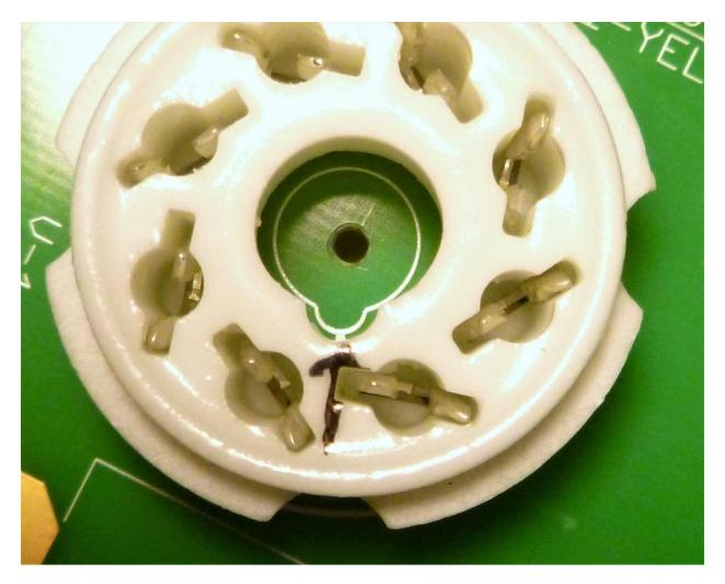
Insert the socket pins into the board so that the two notches align as shown above.
