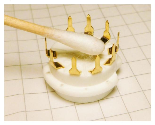
Clean all of the tube socket pins with a solvent-dampened swab.
