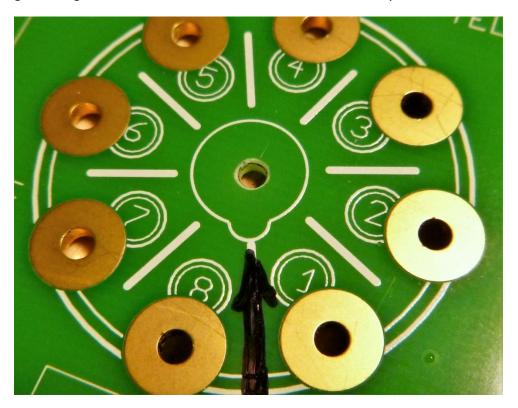
Notice the screened "NOTCH" at the rectifier socket location above, and the notch on the tube socket below.
