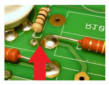
Assemble R106 and R206, both 75K 3W, to the **TOP SIDE** of the board using cardboard spacers. Solder both sides and trim the leads.
