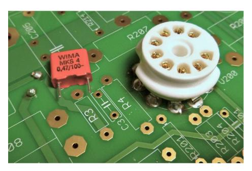
Capacitor C3,  $0.47 \mu F$  100V, can get cramped between resistors R3 and R4 so install it now on the **UNDER SIDE** of the board.
