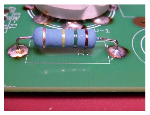
Solder the resistor on **BOTH** sides of the board, trim the leads and remove the cardboard shims.
