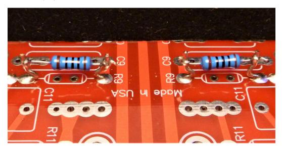
Short lengths of off-cut leads may be soldered to the board as shown above. The resistors then soldered to the leads as shown will allow easier change-out later. If this method is used the off-cut leads must not protrude more than **13mm (1/2")** above the board.
