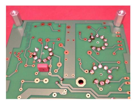
At this point it's a good idea to temporarily install four of the board spacers on the UNDER SIDE at the corners, as shown above. This protects the components once assembled.
