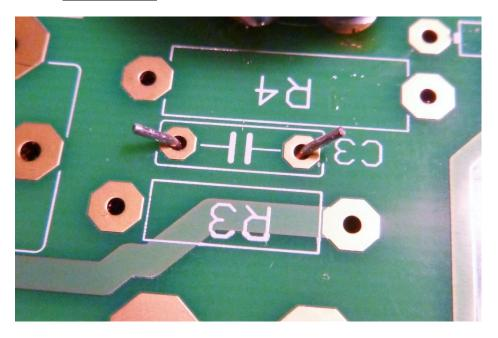
The under side of the board is not labeled but by looking at the top side you can determine if component leads are in the correct holes.
