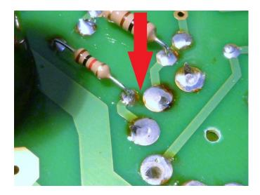
Assemble R101, 1K ¼W, to the **UNDER SIDE** of the board using cardboard spacers. Solder both sides and trim the leads. Be careful to **not** get a solder bridge between R101 and the tube socket pin, **both sides of the board**.
