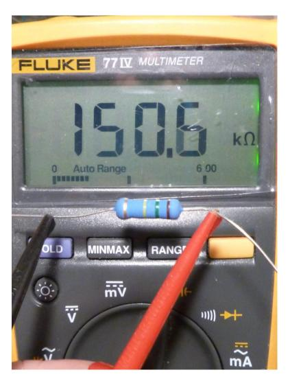
One assembly procedure I can't recommend highly enough is the measurement of **each** resistor before it is assembled to the board.
