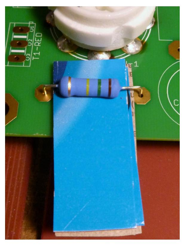
Cut some narrow strips of single wall cardboard, breakfast cereal box or the like, to fashion temporary shims for use between components and the board. Insert at least two shims (using only one shim will make removal difficult) between the resistor and the board.
