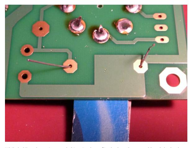
While holding the resistor and shims in place, flip the board over and bend the leads.
