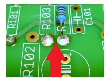
Assemble R104, 5.1K ¼W, to the **TOP SIDE** of the board using cardboard spacers. Solder both sides and trim the leads. Be careful to **not** get a solder bridge between R104 and R103, **both sides of the board**.
