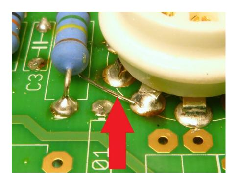
As you work your way through assembling components to the board be mindful of where the cut-off bits of component leads are going. See above. A bit in inadvertent arc welding is not a good thing to have a first start-up.
