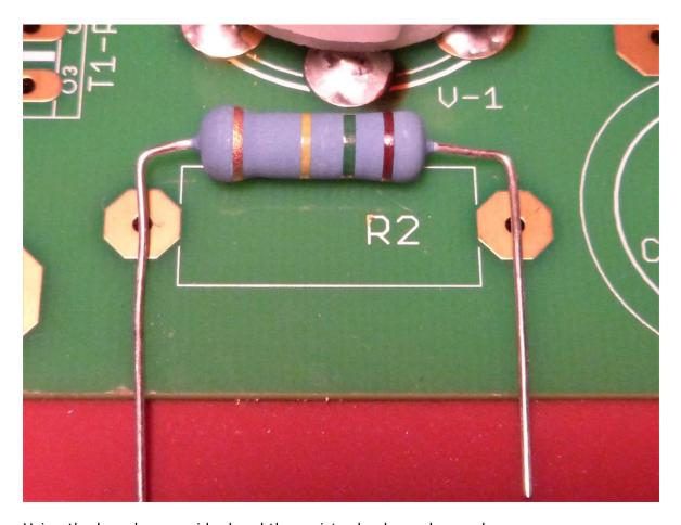
Using the board as a guide, bend the resistor leads as shown above.
