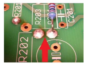
Assemble R204, 5.1K ¼W, to the **TOP SIDE** of the board using cardboard spacers. Solder both sides and trim the leads. Be careful to **not** get a solder bridge between R204 and R203, **both sides of the board**.
