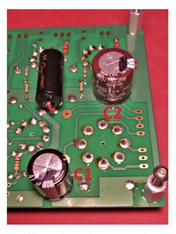
Assemble C1 and C2 to their respective places on the board with the black spots oriented as shown above.
