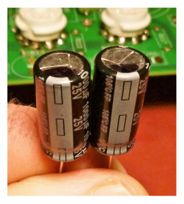
Hold capacitors **C100** and **C200**, both 1,000uF 25V, as shown above. Using a Sharpie marker make a black spot on the tops adjacent to the NEGATIVE stripes.
