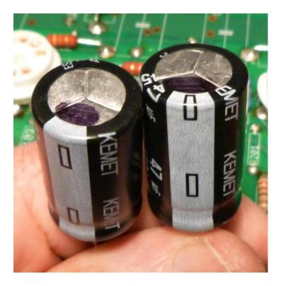
Hold capacitors **C102** and **C202**, both 47uF 450V with thin wire leads, as shown above. Using a Sharpie marker make a black spot on the tops adjacent to the NEGATIVE stripes.
