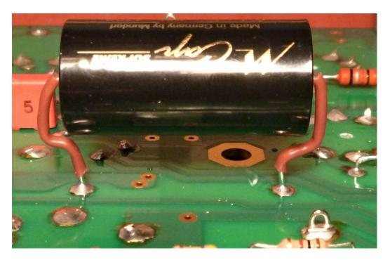
Inset one of the prepped coupling caps into position **C103** as shown above. Solder to the board then turn it over and solder the other side as well. This is especially important as soldering on both sides protects the board traces from damage. Trim the leads.
