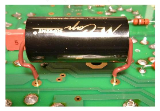
This will necessitate raising the caps clear of the board with the leads bent down and underneath as shown above.
