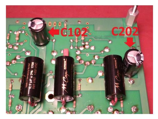
Assemble the caps to the board with the black spots oriented as shown above.
