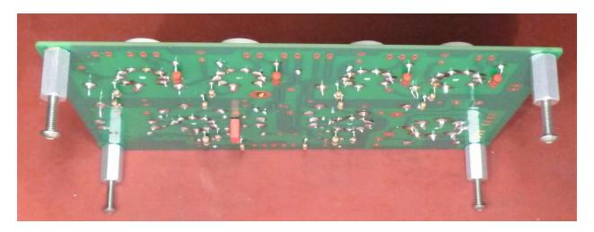
If you have some long 8-32 screws temporarily assemble them to the board spacers. This will protect the coupling capacitors from damage.
