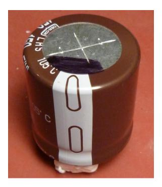
Position capacitor  ${\bf C2}$ , 150uF 450volts as shown above. Using a Sharpie marker make a black spot on the top adjacent to the NEGATIVE stripe.
