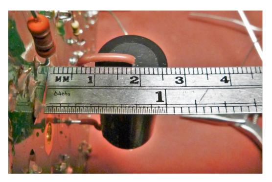
When assembled and soldered to the board the tops of the caps should not protrude more than 28mm (1 1/8") from the board.
