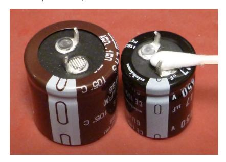
Wipe the pins on both with a solvent-dampened swab.
