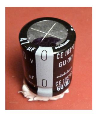
Position capacitor **C1**, 47uF 450volts, as shown above. Using a Sharpie marker make a black spot on the top adjacent to the NEGATIVE stripe.
