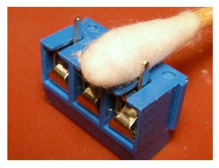
Wipe the terminal block pins with an alcohol-dampened swab.
