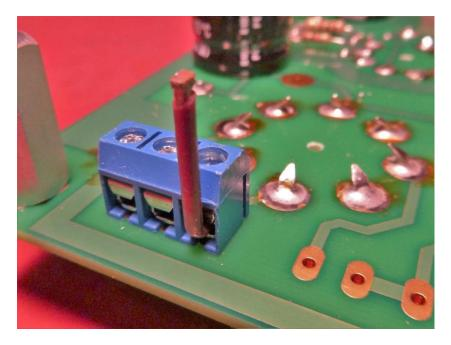
Loosen a screw in the terminal block, insert the tool, tighten the screw then assemble the block to the board.
