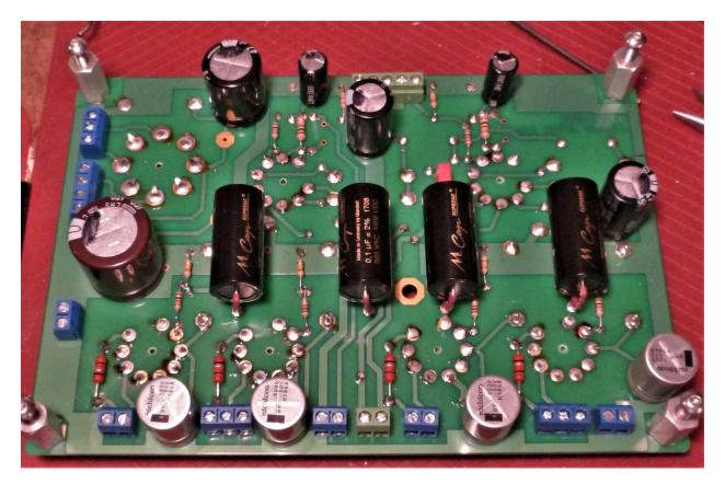
Work your way around the board inserting 2, 3, 4 or 5-pin blocks as required. I've used green ones and blue as seen above, just for the hell of it.
