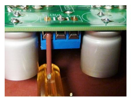
Flip the board over and prop the tool against something to press the terminal block against the board. Solder the terminal pin to the board then move the tool to the next terminal and repeat the procedure. Yes, it's a bit time consuming.
