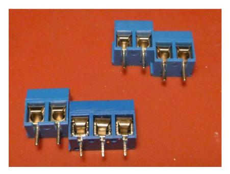
To make a 4-terminal block slide two 2-terminal blocks together.
