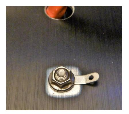
Remove the nut securing the power transformer that's on the bare spot. Hold the screw in place, assemble the solder lug, reassemble the nut and tighten securely.
