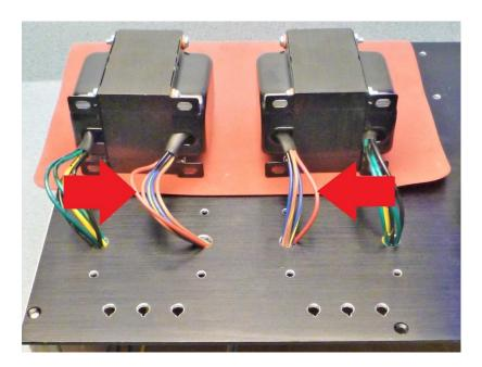
Prep the output transformers with shrink tubing and assemble to chassis with the bundles containing the red wire facing in. Secure with screws, washers and nuts similar to the manner done on the power transformer.
