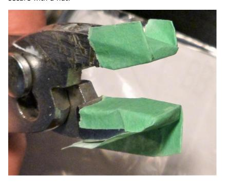
To avoid scratching the top surface apply a layer of tape to your pliers before tightening the nut.
