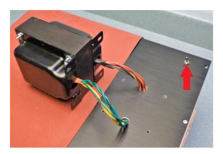
Lay the power transformer on a mat or other protective material as shown above. The bundle with the red wires should be closest to the power switch. Feed the wires through the holes.
