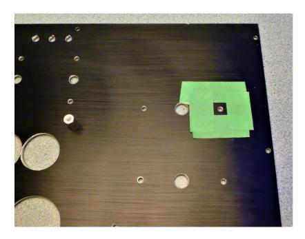
On the  $\underline{\text{under-side}}$  of the top panel mask off a spot about 12mm (1/2") square on the power transformer bolt hole as shown above.
