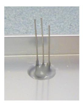
Clean the LED and its hole in the front panel with alcohol. Place the LED in the hole, mix some 5-minute epoxy and spread around the LED. Set aside for several hours to ensure a full cure.
