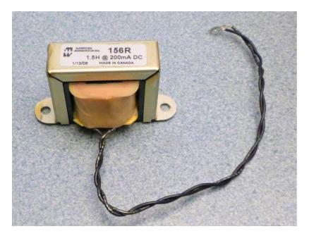
Twist the wires on the filter choke as shown above.
