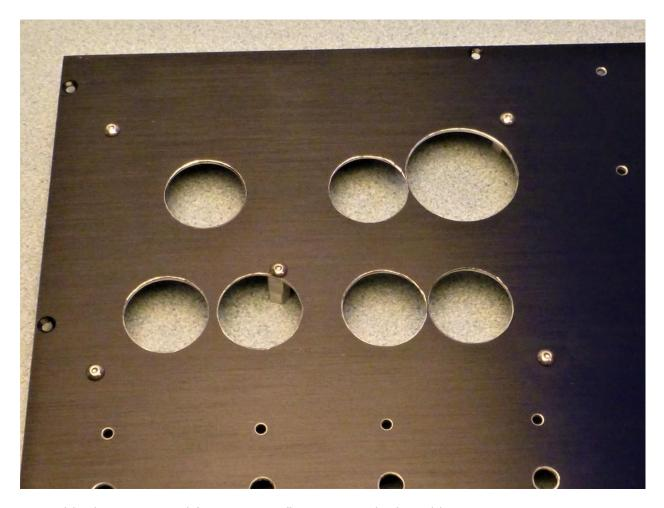
Assemble the screws and five 8-32 x  $34^{\prime\prime}$  spacers to the board locating positions.
