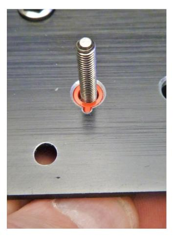
With the rear or the top panel facing you, start from the left, place a red post in the hole with the tab in the notch.
