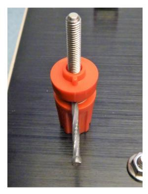
Place a nail through the hole in a speaker binding post and tighten the post. This will prevent distortion of the plastic body in the following steps.
