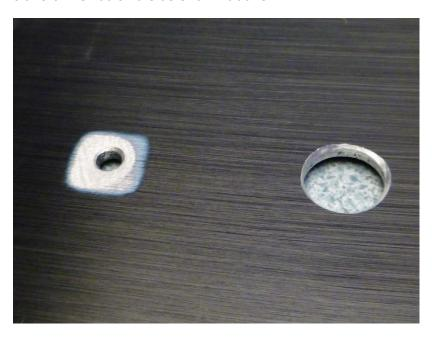
Sand through to bare metal, remove the tape and clean with solvent.
