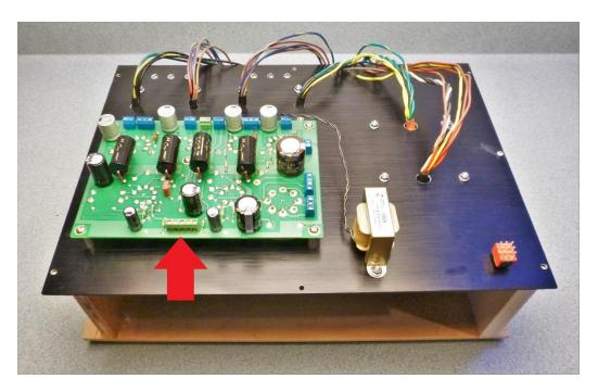
Place the circuit board over the spacers with the 5-terminal connector oriented as shown.
