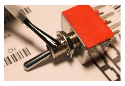
Prep the power switch as shown, apply nail polish to the thread, assemble to top panel and secure with a nut.
