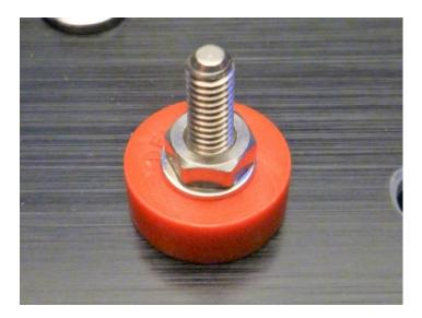
Place the plastic spacer and flat washer over the threaded post. Assemble the nut and tighten securely WHILE grasping the nail to prevent the binding post from rotating.
