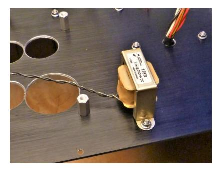
Assemble the choke to the UNDERSIDE of the top plate as shown above. Secure with screws and nuts in manner similar what was done with the transformers.
