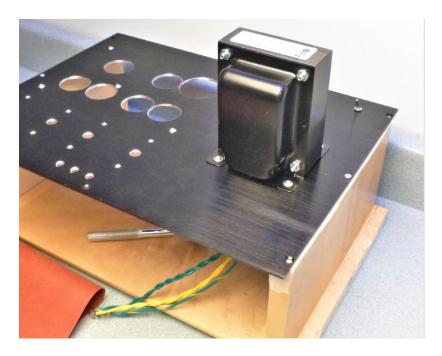
Stand the transformer up sliding the wires through the holes. Assemble four flat washers to four 8-32 or M4 screws. Apply nail polish to the threads. Assemble the screws through the transformer and top plate. Assemble a flat washer and nut to each screw and tighten. If using flanged screws and nuts, flat washers aren't needed.
