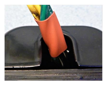
Slide the two pieces of shrink tube over the wires from the power trannie, one at each end. The tubing should go up inside the trannie a bit as shown above. Heat shrink both. The shrink tubing helps protect the wires from chafing on the chassis holes.
