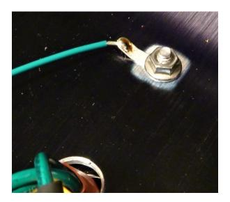
Connect and solder one or the **125mm** wires to the lug under one of the power transformer retaining nuts.
