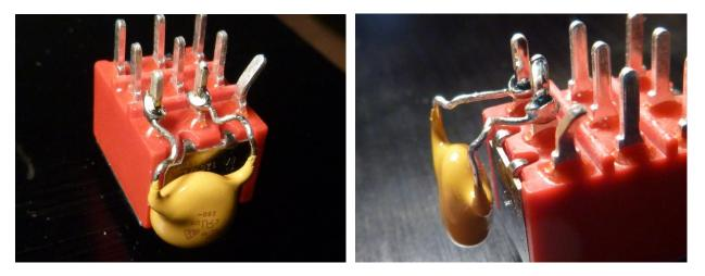
Form the leads of the yellow capacitor and attach to the centre and one side lug of the power switch.
