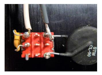
Wrap the white transformer lead around the lug and solder as shown above.
