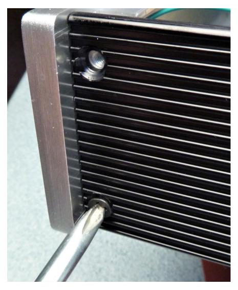
In the following steps put a drop nail polish on the screw threads before assembling.
