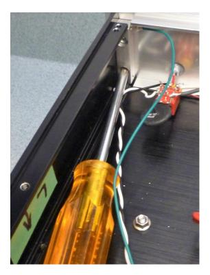
Remove the bottom panel and tighten the screws securing the blocks to the front panel. Place a big drop of nail polish between the block and the head of each screw.
