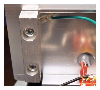
Assemble the connecting block to the front panel at the LED end as shown above. Leave the screws slightly loose.
