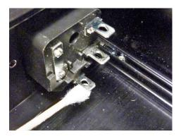
Wipe all three lugs on the AC inlet with an alcohol moistened swab.
