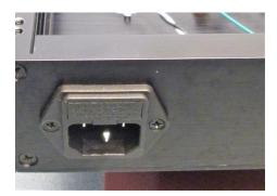
Assemble the AC inlet to the rear panel.
