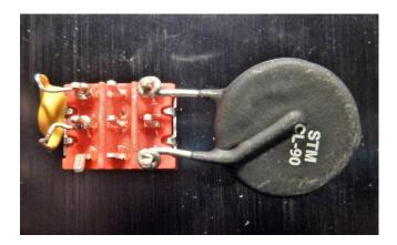
Assemble the Inrush Limiter as shown above, to the two OUTSIDE lugs at the other end of the switch.
