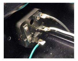
Strip **9mm** from the other end, attach to the lugs of the power inlet as shown and solder. Be careful to not apply heat any longer than necessary. Form the pairs of wires from the input jacks along the side panel, around the front and over to the terminal block connections
