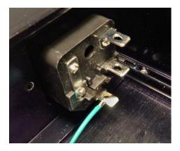
Connect an end of the second **125mm** wire to the ground lug of the AC inlet and solder.
