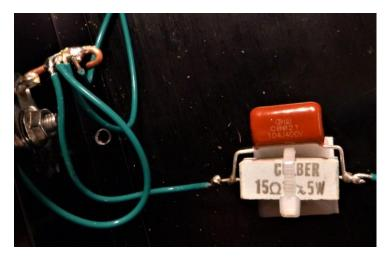
Cut the green lead from connector **28** on the circuit board close to the grounding bar as shown above.
