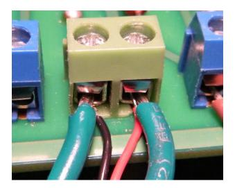
Fully loosen the screws on connector positions 8 and 9.
