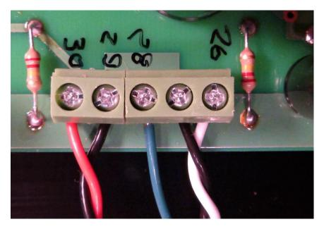
Strip 6mm insulation from the end of each wire and fuse with solder.
