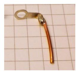
Using a piece of solid copper wire about **30mm** (11/4'') long and a lug, make a grounding bar like the one shown above.
