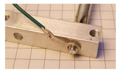
Assemble a screw to one of the side-to-front panel connecting blocks.
