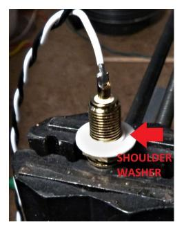
Secure the left channel (back ring) RCA jack in a vise or clamp.
