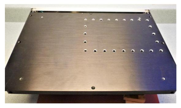
Drop the bottom panel in place to ensure it fits between the side panels.
