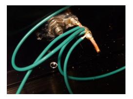
Wrap all 4 ends of the green grounding wires around the grounding bar and solder.
