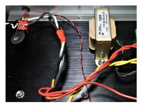
Fold the unused primary wire back on the other wires. Insulate and secure with a piece of tape. We'll have a more secure solution once the final primary selection is made during testing.
