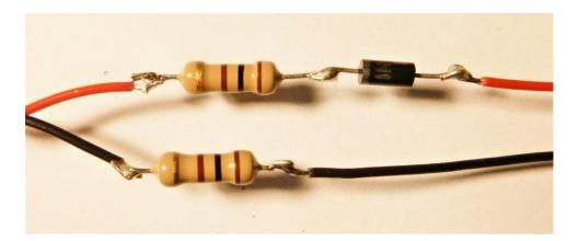
Strip the ends of the wires coming from the LEDs, connect to the resistors as shown above and solder the connections.
