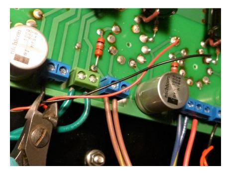
Run the wires along the rear of the circuit board and trim as shown above. Save the offcut ends.
