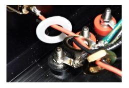
Slide both jack-wire combinations through the holes in the rear panel from the **outside**. Slide, in this order, the flat plastic washer, the ground lug and the nut as shown above. Push the washer and lug over the nut then only <u>start</u> the nut on the jack.
