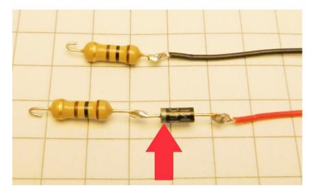
Prep, connect and solder two  $100\Omega$  resistors and the 1N4007 diode as shown above to the red and black offcut ends. Note the location of the band on the diode.
