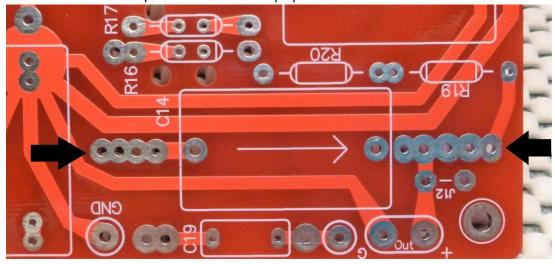
We must be careful to get the components on the correct side of the PCB. To put the tube sockets on the wrong side would mean a nasty repair.
