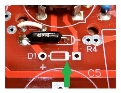
Install the diodes with its white band in the same orientation. Too much heat during soldering can damage diodes. By bending the leads to space them up off of the board, as shown below, a bit of length is gained between the solder site and the diode.
