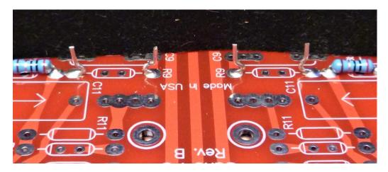
Solder the desired resistor to the protruding leads. It may be changed more easily.
