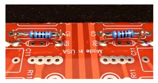
Assemble R10, two places to the board but space above the board 1 to 2mm. Solder and trim.
