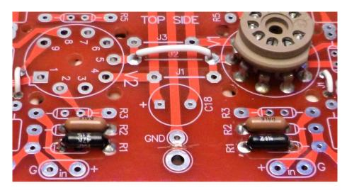
Assemble R3, R4 and R5 to the board in their respective positions. Solder and trim the excess lead lengths.
