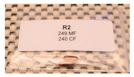
Assemble resistors R2, two places, to the board as shown below, solder and trim the excess leads.
