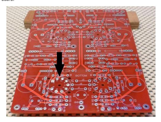
Flip the board over and solder the socket on the top side as well. This will be more secure when inserting and removing tubes.
