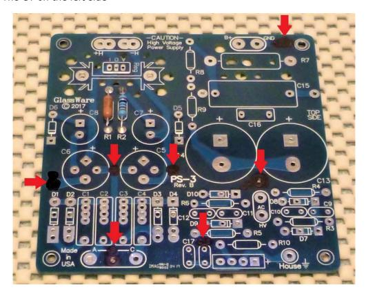
Assemble D5 and D6 to the board with the banded ends in the orientation shown below. Keep them about 2 to 3mm above the board to lessen their heating when soldering.
