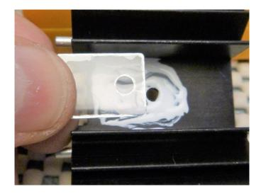
Spread a bit of heatsink compound on the back of the LD1085 regulator.
