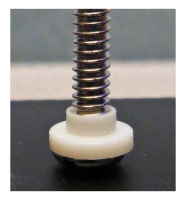
Assemble the screw and washer to the reg and heatsink as shown.
