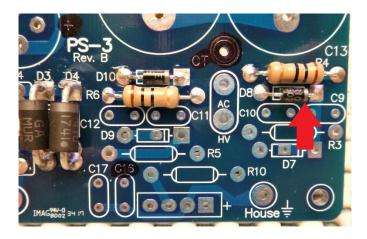
Assemble caps C9, 10, 11 & 12 to the board in the positions shown below. Solder and trim.
