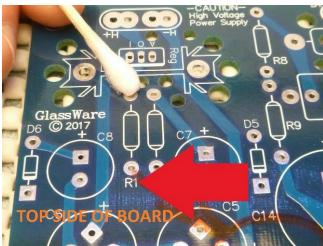
Place the board on your bench as shown below. The circled **PS-3** should still be there from the chassis layout performed earlier. The **Made in USA** should be on the lower left and **House** on the right. Assemble R1 to the board, solder both sides and trim the leads.
