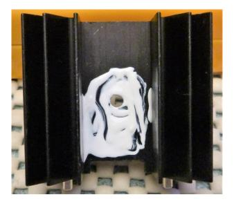
Put the insulator, shown below, on to the heatsink so that the hole in each aligns with the other.
