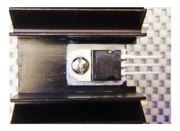
Optional: Even though the solder mask on the board insulates the traces and the anodizing on the heat sink is an insulator I like to go one step farther. I like to put a few thin strips of kapton tape near the pins on the heatsink, see below. Cellophane tape would work as well.
