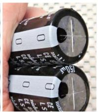
Assemble C5 & C6 to the board with the negative sides facing the C1 – C4 caps as shown below. Solder and trim the leads.
