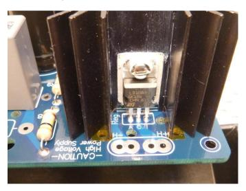
Solder the pins of the heatsink and the regulator to the board.
