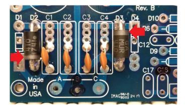
Assemble D1 & D4 to the board with the bands in the orientation shown. Keep them 2 to 3mm above the board. Solder and trim.
