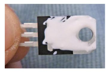
Assemble the LD1085 reg to the heatsink so the holes align.
