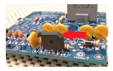
Assemble caps C15 and C16 to the board. Solder and trim.
