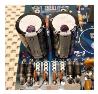
Assemble C7 & C8 to the board with the negative sides facing C5 & C6 as shown below. Solder and trim the leads.
