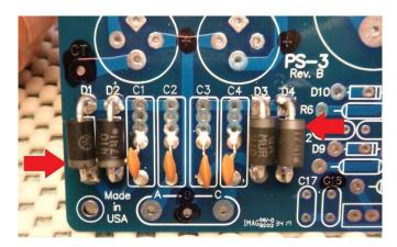
Assemble D10 to the board with the band in the orientation shown. Keep it 2 to 3mm above the board. Assemble R4 to the board. Solder both and trim.
