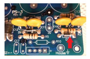
Assemble R10 and C17 to the board, solder and trim.
