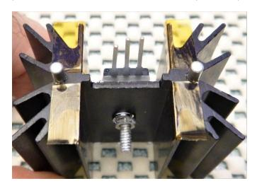
Assemble the heatsink/regulator combination to the board. Guide the regulator pins into the board first then the heatsink pins.
