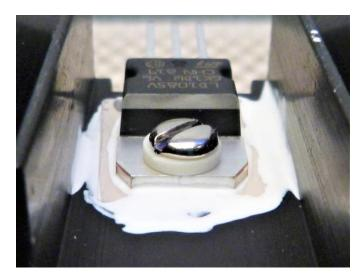
Assemble the lock washer and nut to the screw. Tighten and keep the reg parallel to the heatsink walls as shown.
