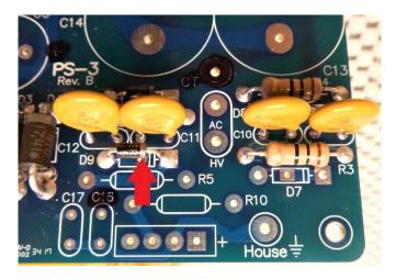
Assemble D7 to the board with the band in the orientation shown. Keep it 2 to 3mm above the board. Assemble R5 to the board. Solder both and trim.
