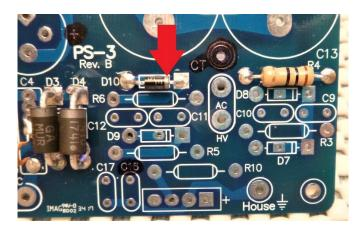
Assemble D8 to the board with the band in the orientation shown. Keep it 2 to 3mm above the board. Assemble R6 to the board. Solder both and trim.
