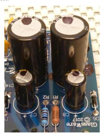
As received the pins on C13 and C14 are bent. Straighten them to allow easier board insertion.
