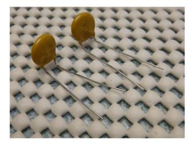
Insert them through the switch side of the board and solder both sides as shown below. Trim the leads.
