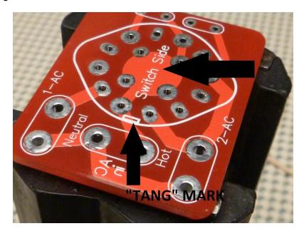
Assemble the switch to the board with the locating "TANG" on the switch positioned as shown.
