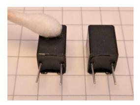
Wipe the **bottom** of the board in the areas around C14 as shown below.
