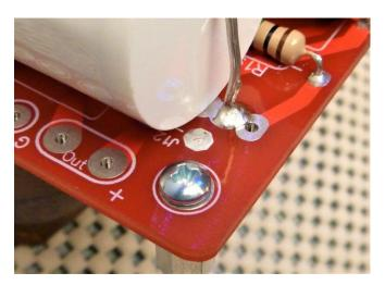
Assemble capacitor C17 to the board.
