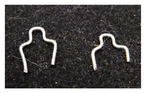
Install on the <u>bottom</u> of the board at position J12, two places, as shown below. Trim the excess protruding from the <u>top</u> side of the board then solder. These jumpers and caps C19 are installed on the bottom because the main output caps, C14, require as much space as possible on the top side of the board.
