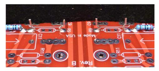
Solder the desired resistors to the protruding leads. It may be changed more easily.
