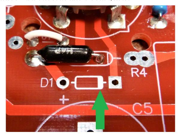
Install the diodes with its white band in the same orientation. Too much heat during soldering can damage diodes. By bending the leads, as shown below, a bit of length is gained between the solder site and the diode.
