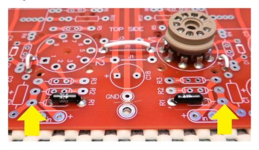
Do not use the R2 resistors supplied with the kit. Use the 200 ohm resistors purchased separately.
