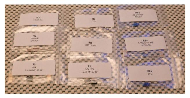
Open the package containing the two R1s (one for each channel) and check resistance with a multimeter.
