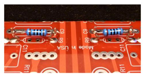
Assemble R10, two places to the board <u>but space above the board 1 to 2mm.</u> Solder and trim.
