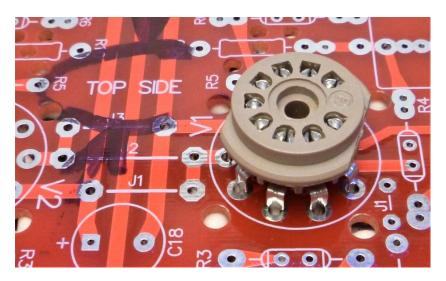
Flip the board and socket over, rest in on your bench and prop the far end up with wood blocks or similar to keep the board parallel to the top face of the socket. Solder the socket to the board.
