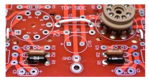
Assemble R3, two places, to the board. Solder and trim the excess lead lengths.
