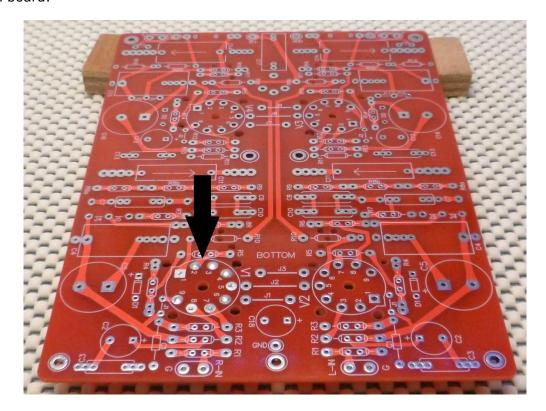
Flip the board over and solder the socket on the top side as well. This will be more secure when inserting and removing tubes.
