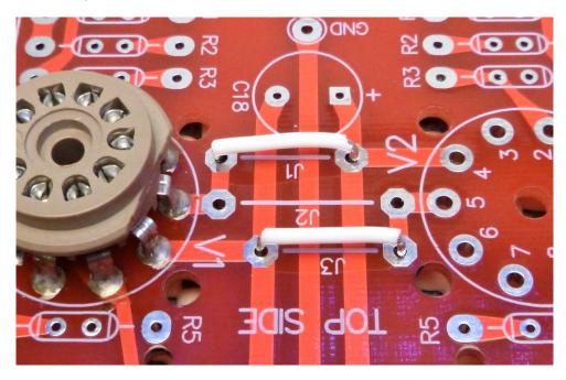
Note, there are three J1s on the board, 2 for grounding and one for filament supply. The two J1s close to the two R4s are **not** used with 12AT7 input tubes.
