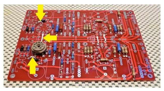
Install the remaining tube sockets, first cleaning the socket pins with alcohol. Solder the socket pins on both sides of the board.
