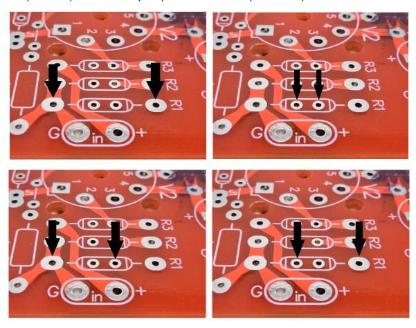
The resistors are packaged with the required value by circuit location. All the same it pays to check them with your multimeter before assembling to the board.
