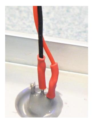
Place heat shrink over the connections. Twist the wires together. Set the front panel aside.
