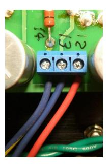
Connect the **red** wire **from the transformer** to terminal **12**.
