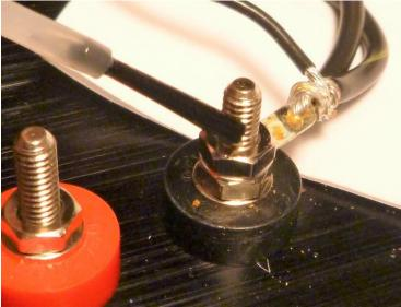
Spin the nuts down to press the lugs against the first nut.
