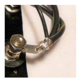
Place solder lugs over the BLACK connector posts on both channels and start a nut to keep it on. The nut will be tightened later after soldering.
