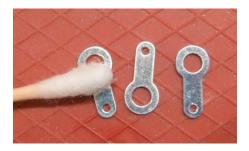
Wipe all six terminal lugs supplied with the speaker terminals with alcohol.
