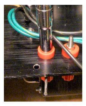
Using a nail to prevent twisting of the speaker terminals, re-tighten the nuts securing the terminals to the top panel.
